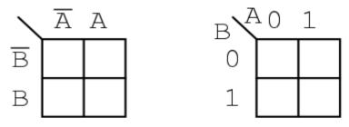
We don't waste time drawing a Karnaugh map like (c) above, sketching a simplified version as above left instead. The column of two cells under A' is understood to be associated with A', and the heading A is associated with the column of cells under it. The row headed by B' is associated with the cells to the right of it. In a similar manner B is associated with the cells to the right of it. For the sake of simplicity, we do not delineate the various regions as clearly as with Venn diagrams.
