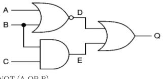
D = NOT (A OR B)E = B AND C Q = D OR E = (NOT (A OR B)) OR (B AND C)
