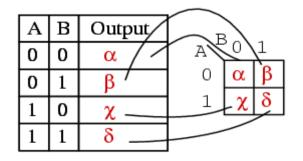
The outputs of a truth table correspond on a one-to-one basis to Karnaugh map entries. Starting at the top of the truth table, the A=0, B=0 inputs produce an output  $\alpha$ . Note that this
