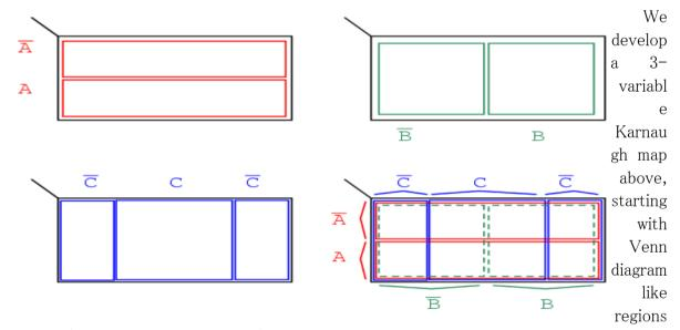
. The universe (inside the black rectangle) is split into two narrow narrow rectangular regions for A' and A. The variables B' and B divide the universe into two square regions. C occupies a square region in the middle of the rectangle, with C' split into two vertical rectangles on each side of the C square.
